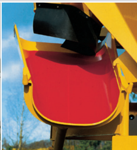
Wear protection in the pivoting discharge chute.
