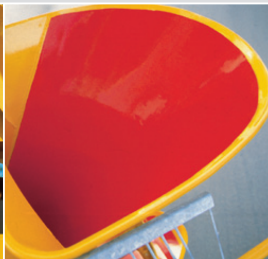
Wear protection in the inlet hopper.
